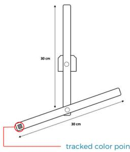
To build a chaos pendulum, only two pendulums rods have to be coupled together, so that the second pendulum can behave chaotically. However, this choice also has some disadvantages: Although the centrifugal force turned out to be negligible at the frequencies examined, there is a problem with the representation and evaluation. For the dimension  $D$  of the phase space of a system with  $n$  degrees of freedom the following applies:
